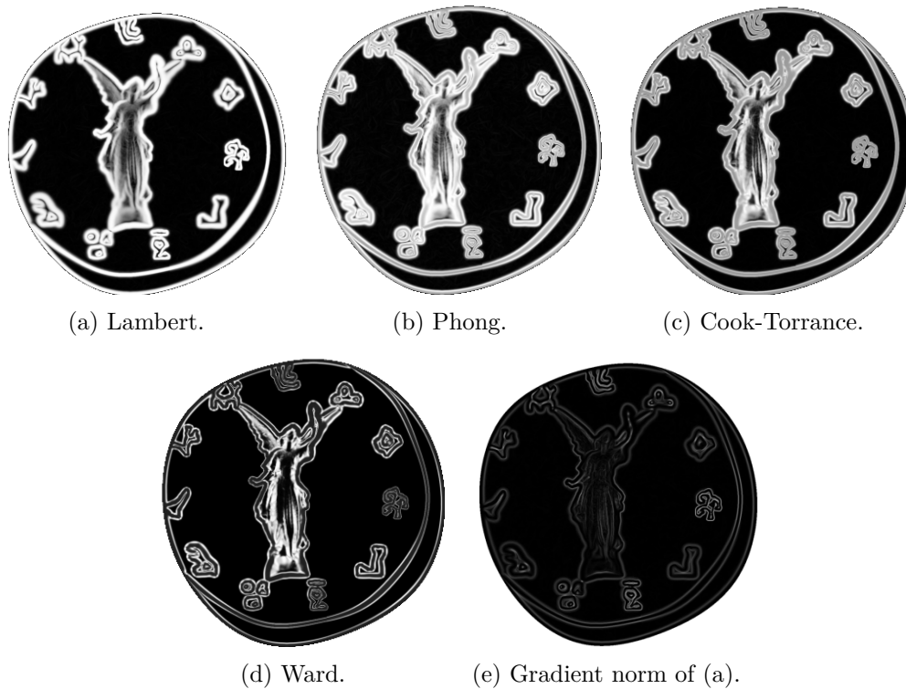
Figure 2.32: Energy maps for four types of BRDFs with increasing specularities and gradient magnitude of the Lambertian energy map.
