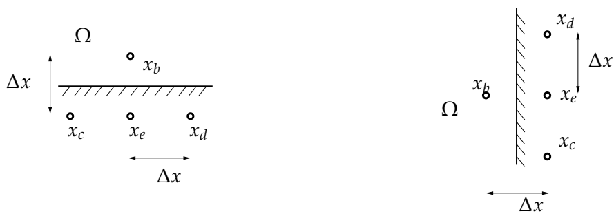
Figure 2: Left : Boundary node x_b in the bottom of the domain \Omega . Right : Boundary node x_b in the right of the domain \Omega .
