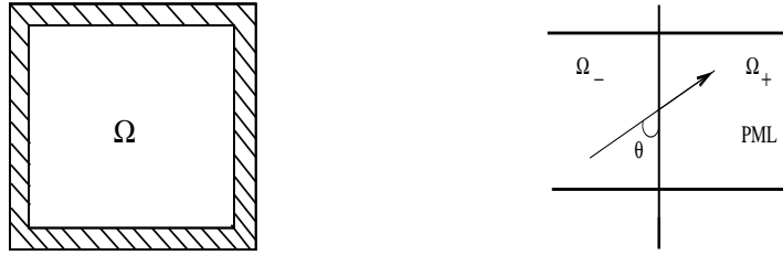
Figure 1: Left : Domain of interest \Omega and buffer/sponge domain (PML), Right : Interface : \Omega_- acoustics domain / \Omega_+ PML domain
